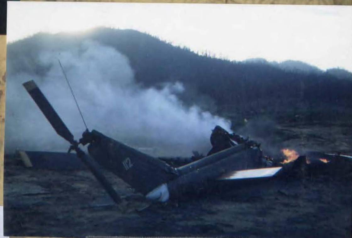
June 1969 Damaged Huey landed at Firebase Bastonge; CH-47 Chinook was lifting Huey back to Phu Bai but dropped it at pickup location. Electrical short caused fire upon impact.
