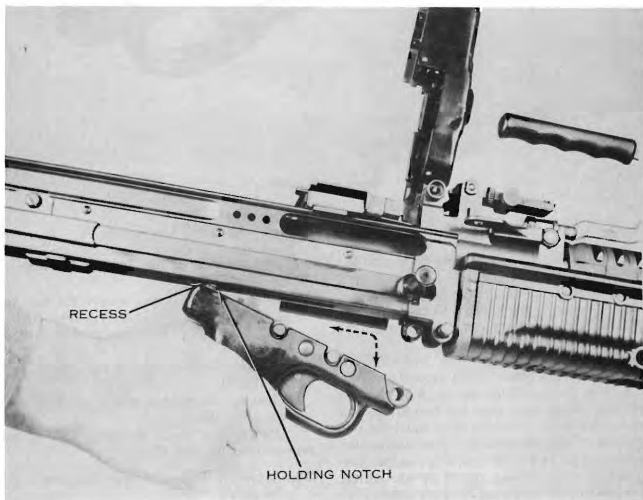
Figure 10. Removing the trigger housing group.
