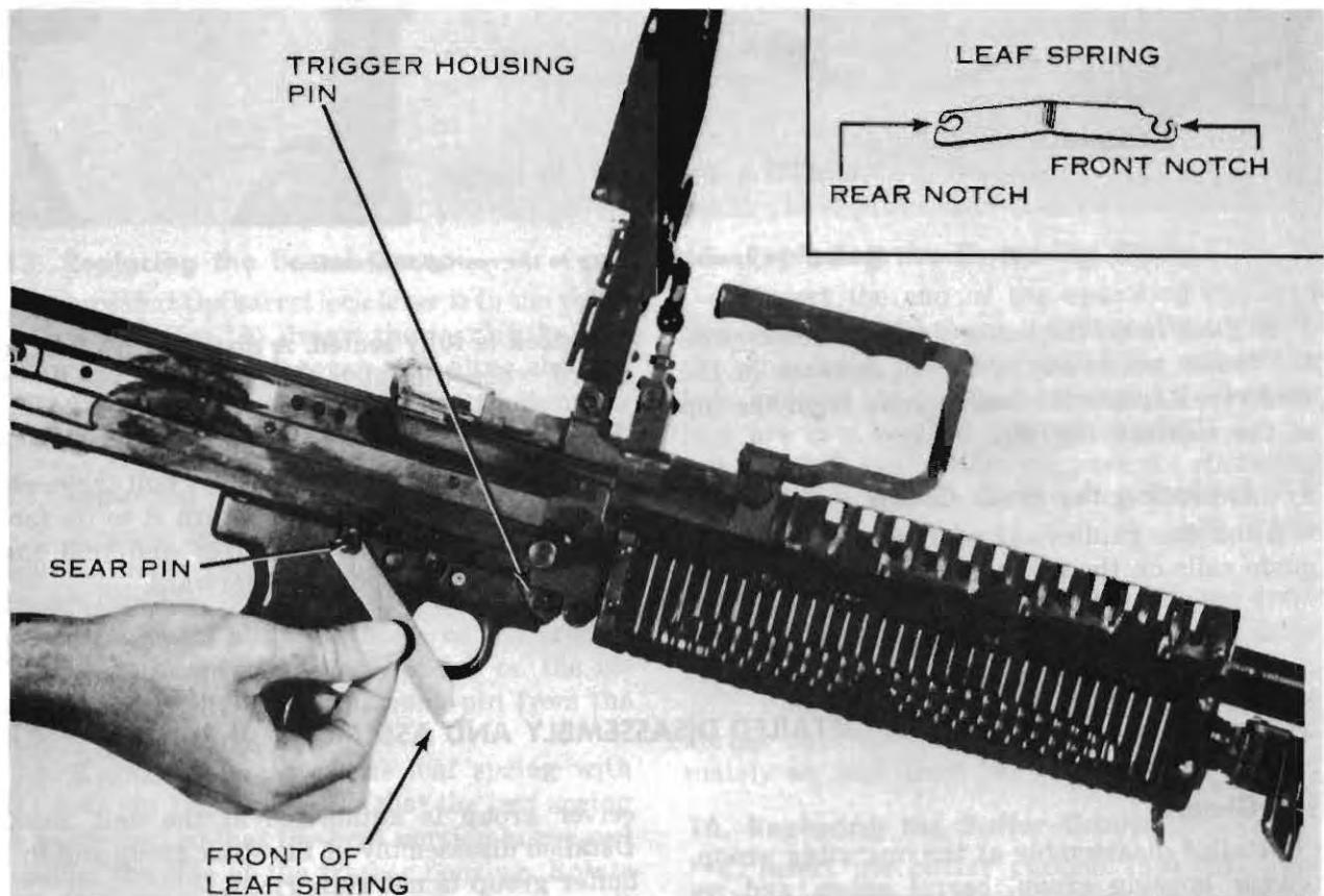
Figure 9. Removing the leaf spring.
