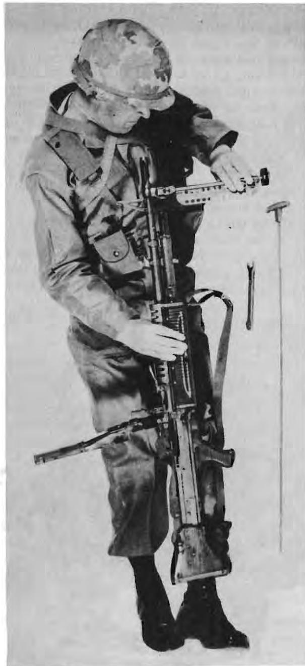
Figure 54. Gunner inspecting barrel and bleeder hole.
