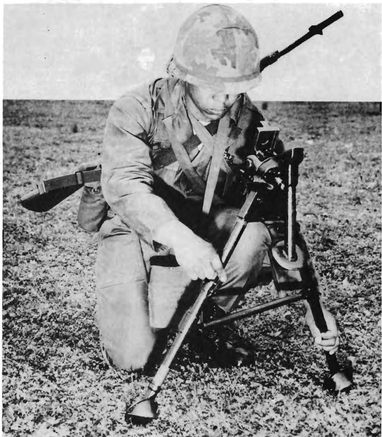
*Figure 69. Closing the tripod legs.*
