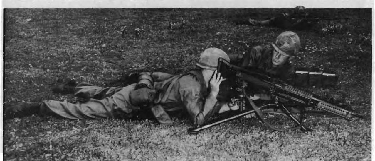
*Figure 65. Attaching the traversing and elevating mechanism.*
