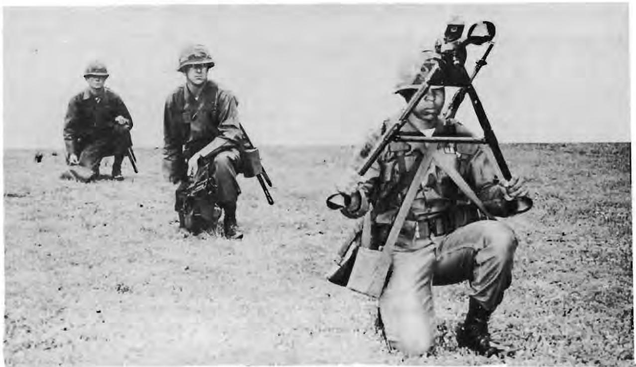
Figure 63. Opening the tripod.
