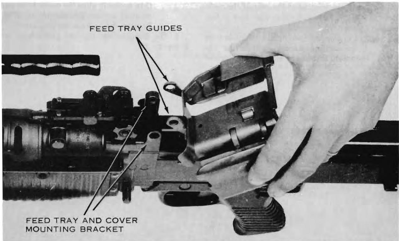
Figure 29. Removing the feedtray.
