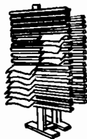
DRYING RACK MADE WITH 2" x 2" UPRIGHTS WITH 1" x 1" CROSS BARS ABOUT AN INCH APART
