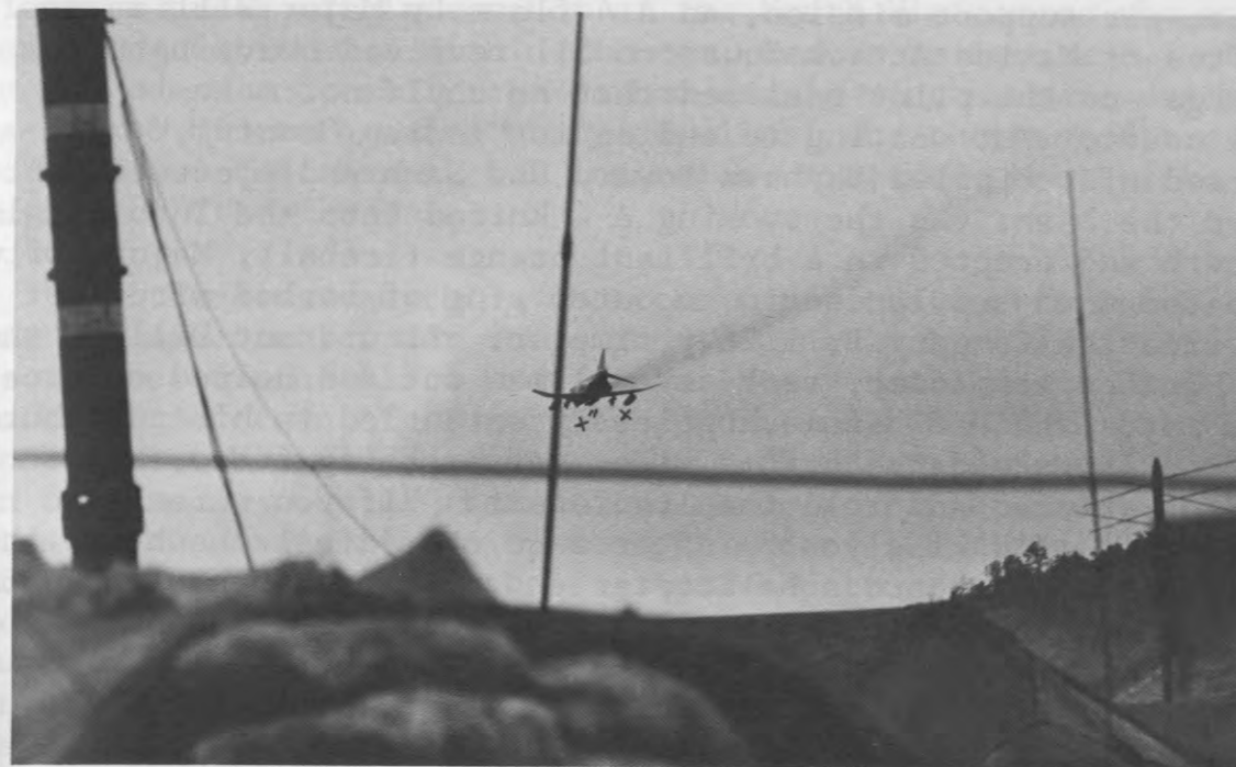
Marine F-4B Phantom delivers Snakeye bombs on enemy trenches. Large tail fins retard the descent of the bombs. (Photo courtesy David D. Duncan)
