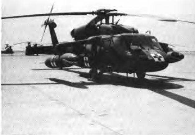
Desert Storm UH60 equipped for long range self-deployment from Germany to Saudi Arabia.
