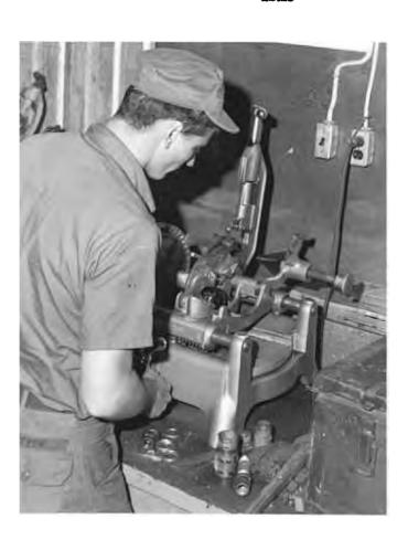
MAINTENANCE MARINES — Lance Corporals Larry C. Fleck (Indianapolis, Ind.) and James A. Thomas (Des Moines, Iowa) repair the yoke on the biped mechanism of an 81mm mortar. The two Leathernecks are attached to the Infantry Weapons Section, Maintenance Bn., Force Logistic Command, near Da Nang. Maintenance Bn. has the capabilities of repairing nearly every piece of combat equipment used by Marines in Vietnam. (OFFICIAL USMC PHOTO by Cpl. Mike Teramoto) 3-0050-67
