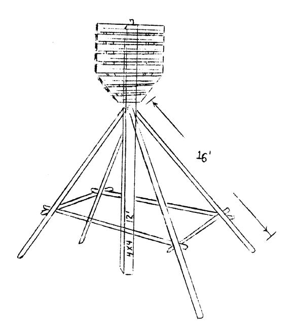
CONSTRUCTED OF WOOD WITH ONE LARGE NAIL EXTENDING FROM THE CENTER POLE. NO WIRES ATTACHED OR LOCATED IN THE AREA.
