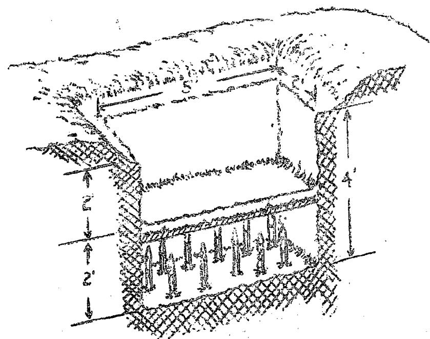
Schematic drawing of Man-Trap (Prone shelter constructed with concealed punji stakes).
