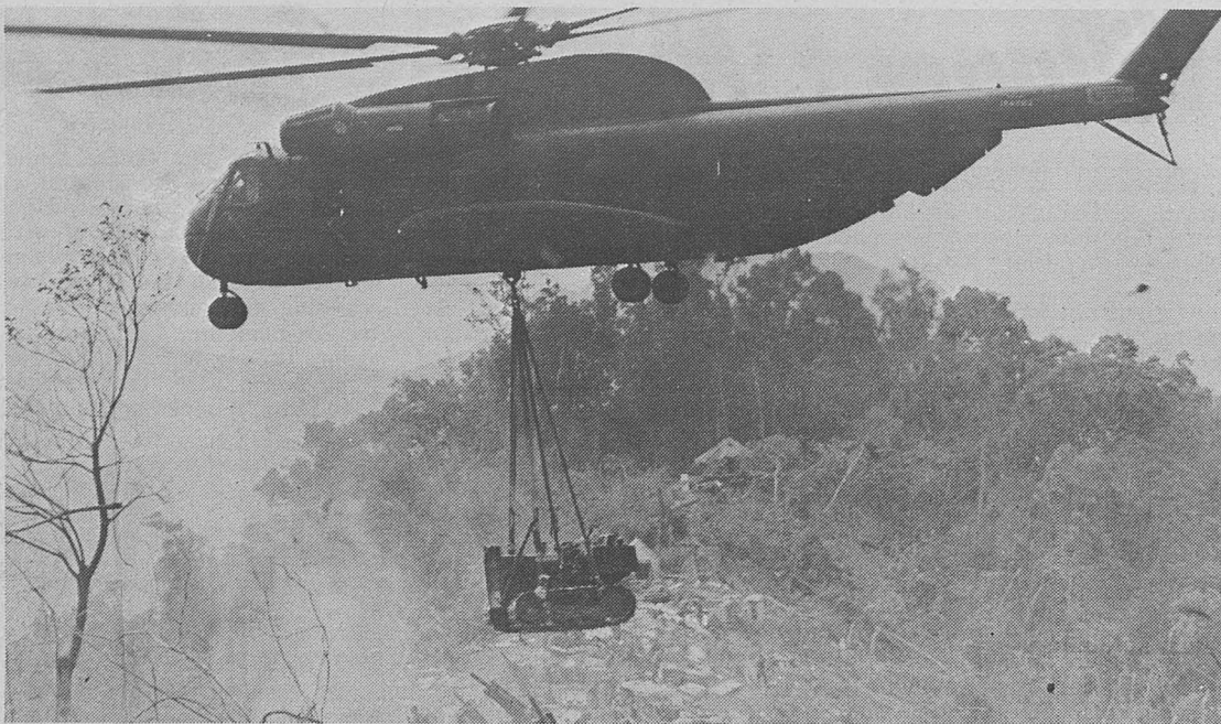
LIFTING POWER —A Marine Sea Stallion helicopter lifts a bulldozer at a fire support base in northern I Corps. The huge choppers make Vietnam's mountain top accessible to Marine ground troops and deliver supplies to sustain the posts.
