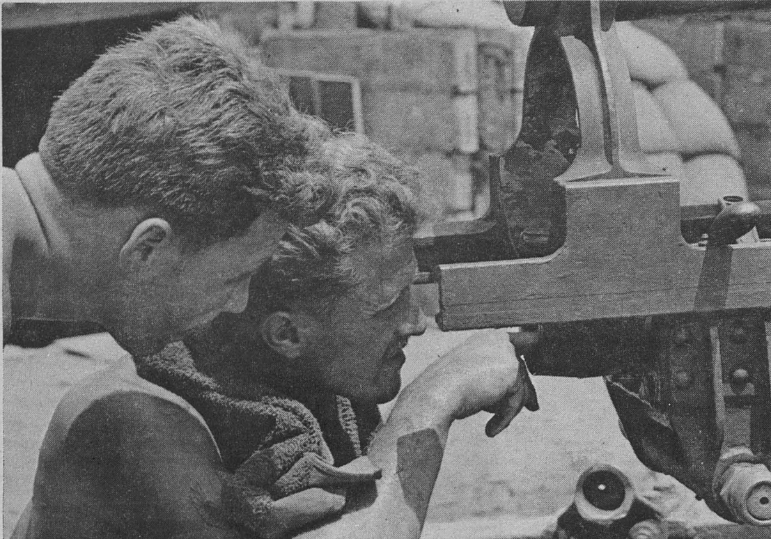
LCPLS DON WHITAKE, left, (7153 Elevloz, Buena Park, Calif.) and Ron Woodward (Kearns, Utah) repair the cradle mechanism on a 105mm howitzer at the An Hoa Combat Base south of Da Nang. The two Marines are attached to the ordnance maintenance section of Force Logistic Support Group Alpha, which is responsible for repair and maintenance of all artillery pieces used by the 11th Marines, 1st Marine Division. (Photo by Sgt. Joe Coder)
