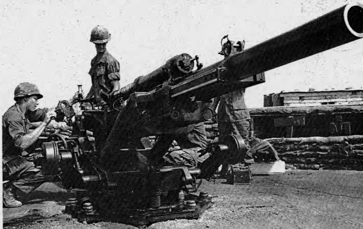
RAMMING THE PROJO —As the gunner sets the deflection and levels the bubbles on the sight, the #1 cannoneer rams the projectile and cannister into the tube. (PHOTO BY 1LT R.S. PERRY)
