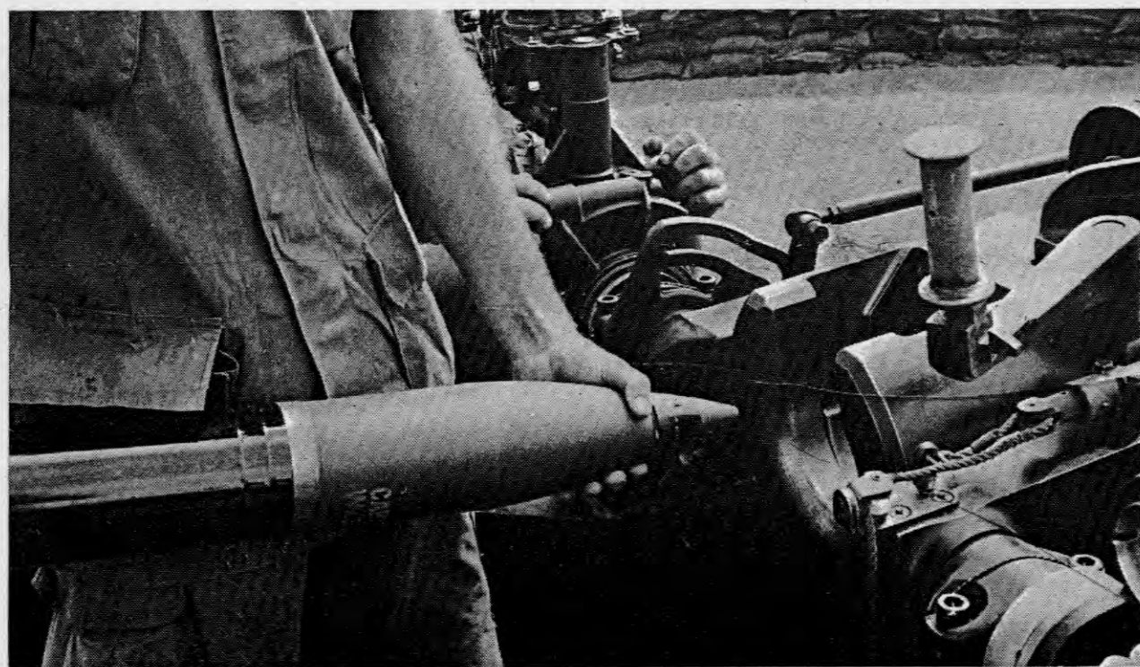
RAMMING THE PROJO —As the gunner sets the deflection and levels the bubbles on the sight, the #1 cannoneer rams the projectile and cannister into the tube. (PHOTO BY 1LT R.S. PERRY)
