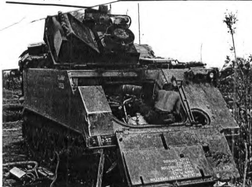
EATEN BY WHAT? —A Regular from the 2nd Battalion (Mech) 22nd Infantry, appears to be swallowed up by his track as he takes out the last remaining screws prior to removing his blown engine. Triple Deuce's new maintenance program has eliminated the delay in sending the tracks to rear areas to be repaired. (Photo by SP4 Dennis Leblanc)
