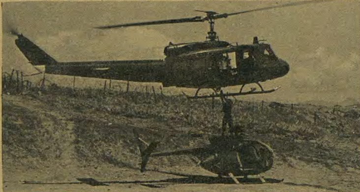
"Gunsmoke Recovery" team rig up this LOH (Light Observation Helicopter) to be transported back of Chu Lai for repair. (U.S. Army Photo)
