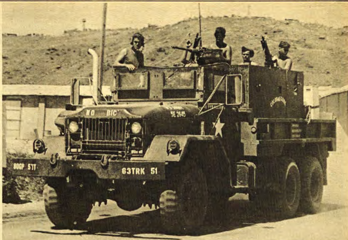
READY WITH PLENTY OF FIREPOWER IS THIS GUN TRUCK from the 63rd Trans. Co. leading another convoy on the hazardous trip on Highway 1. Armed with two 7.62 mm and one .50 cal. machineguns, the truck spells bad news for snipers and ambushers attempting to slow the supply runs made by the 63rd to 11th Bde. bases. (Photo by SP4 Steve Tipton, 11th Bde. IO)
