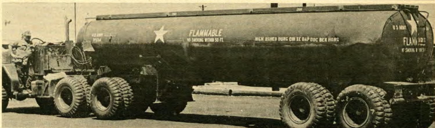
MSG Joe Young proudly displays his creation. At first it appears simply to be an oil tanker, but isn't. Instead the tank carries asphalt for reducing dust on roads and helipads. (Photo by 26th Eng. Bn.)
