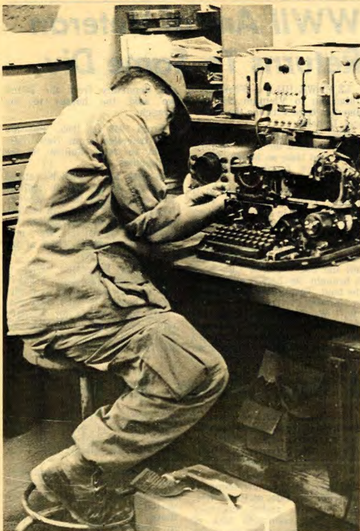
MAKING THE FINAL INTRICATE adjustments to the TT-4 teletype machine is the job of SP5 James Orcutt (St. Paul, Minn.). Thousands of pounds of equipment are repaired monthly by the men of the 723rd Electronic Maintenance Shop. (U.S. Army Photo)
