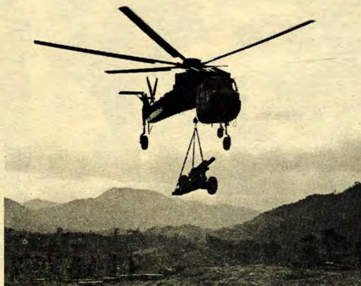
LOWERING ONE OF the 155mm howitzers to a hilltop in New Hau Duc Valley is a CH-54 Sky Crane. The move enabled B Btry., 3-16 Arty. to provide support for allied forces who were sweeping the area. (Photo by PFC Thomas A. Budarz, Divarty IO)
