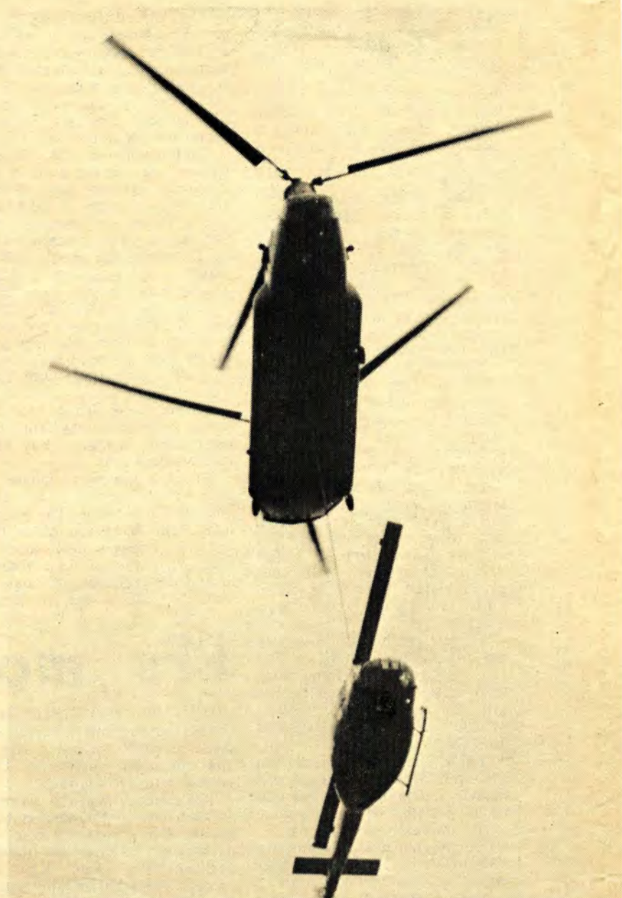
The powerful lift capabilities of the Chinook is illustrated in this photo which shows the hook carrying a Huey chopper which had developed mechanical problems.
