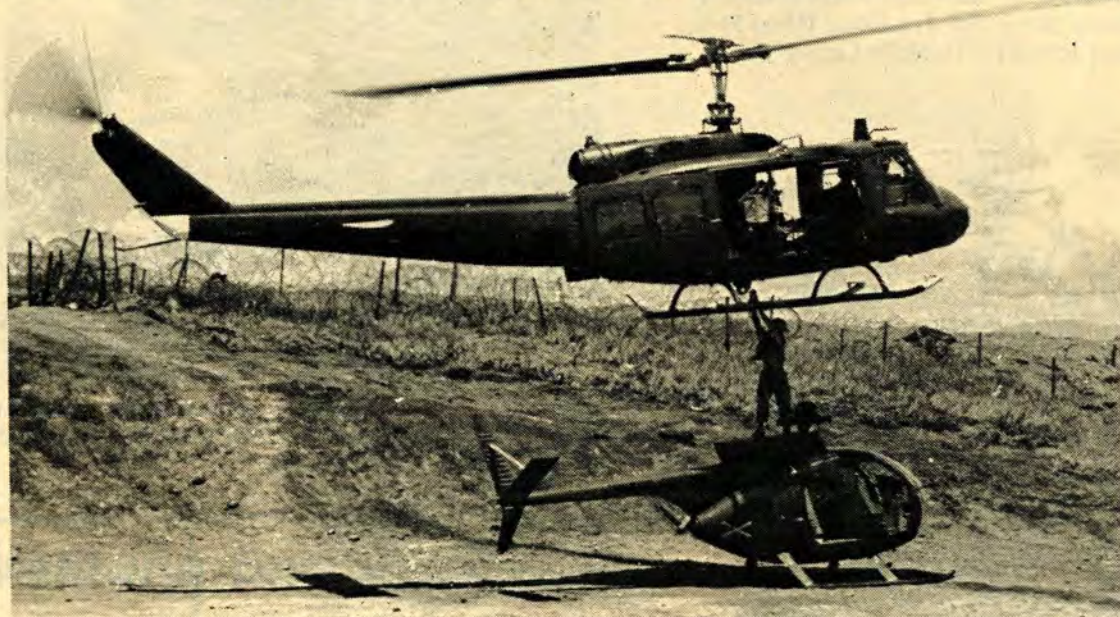
A crew member of the "Huey" rescue ship connects a sling to the main rotor socket of a disabled LOH. The LOH rotor blade was previously removed to facilitate air-removal to Chu Lai. (Photo by SSG Tim Palmer)
