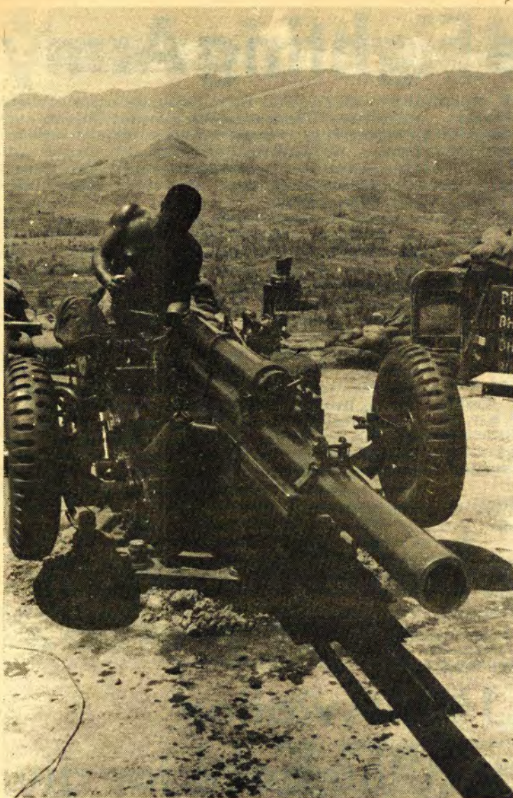
This soldier of the 3rd Battalion, 82nd Artillery runs a maintenance check on a 105mm gun to ensure that it continues to function properly. (U.S. Army Photo)
