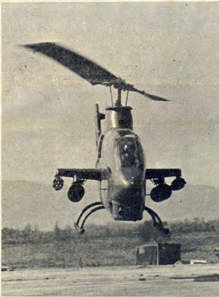
The slender AH-1G (Cobra) gunship, equipped with mini-gun, 40mm grenade launcher and rocket pods, is one of the most effective weapons in Vietnam today. The one in this picture prepares for a mission in the 23rd Infantry Division. (U.S. Army Photo).
