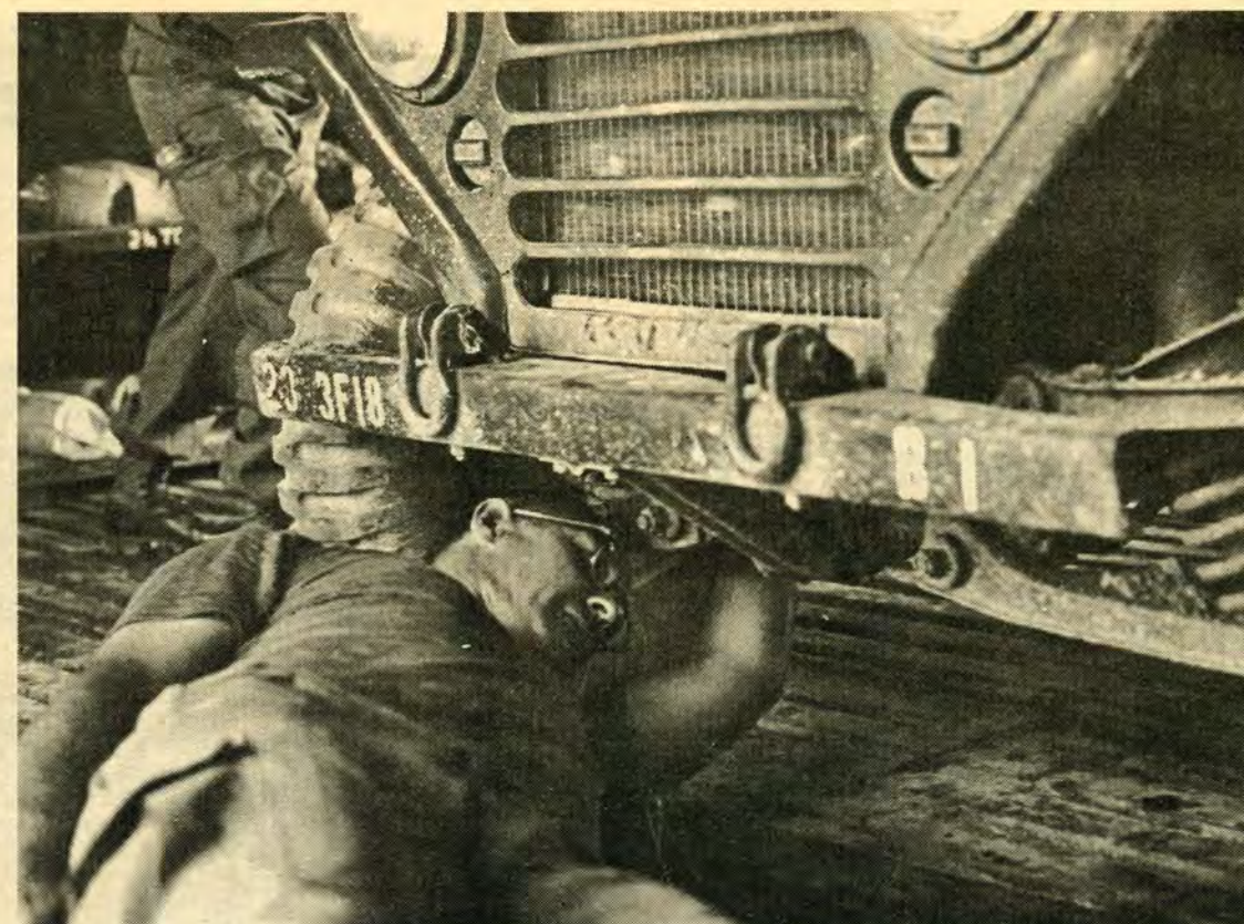
Staff Sergeant Homer L. Jarrell (Logan, Va.), vehicle inspector, checks out the front axle of a jeep at LZ Phoenix where B Battery, 3rd Battalion, 18th Artillery is based at Tien Phuoc. (U.S. Army Photo by SP4 Guy Winkler)
