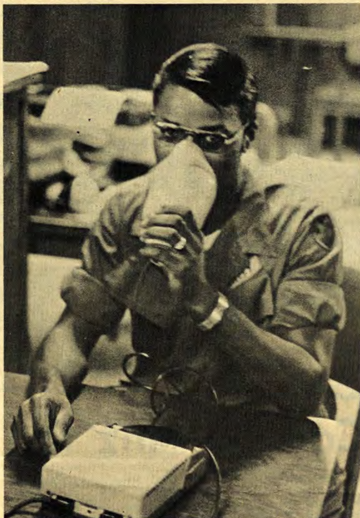
Specialist Six Jack Calhoun (Haverstraw, N.Y.) demonstrates the use of the stenomask, an aid in recording testimony. During trials, a court reporter repeats both questions and answers into the device without interrupting the proceedings. (U.S. ARMY PHOTO BY SP4 SAM ROUSSO)
