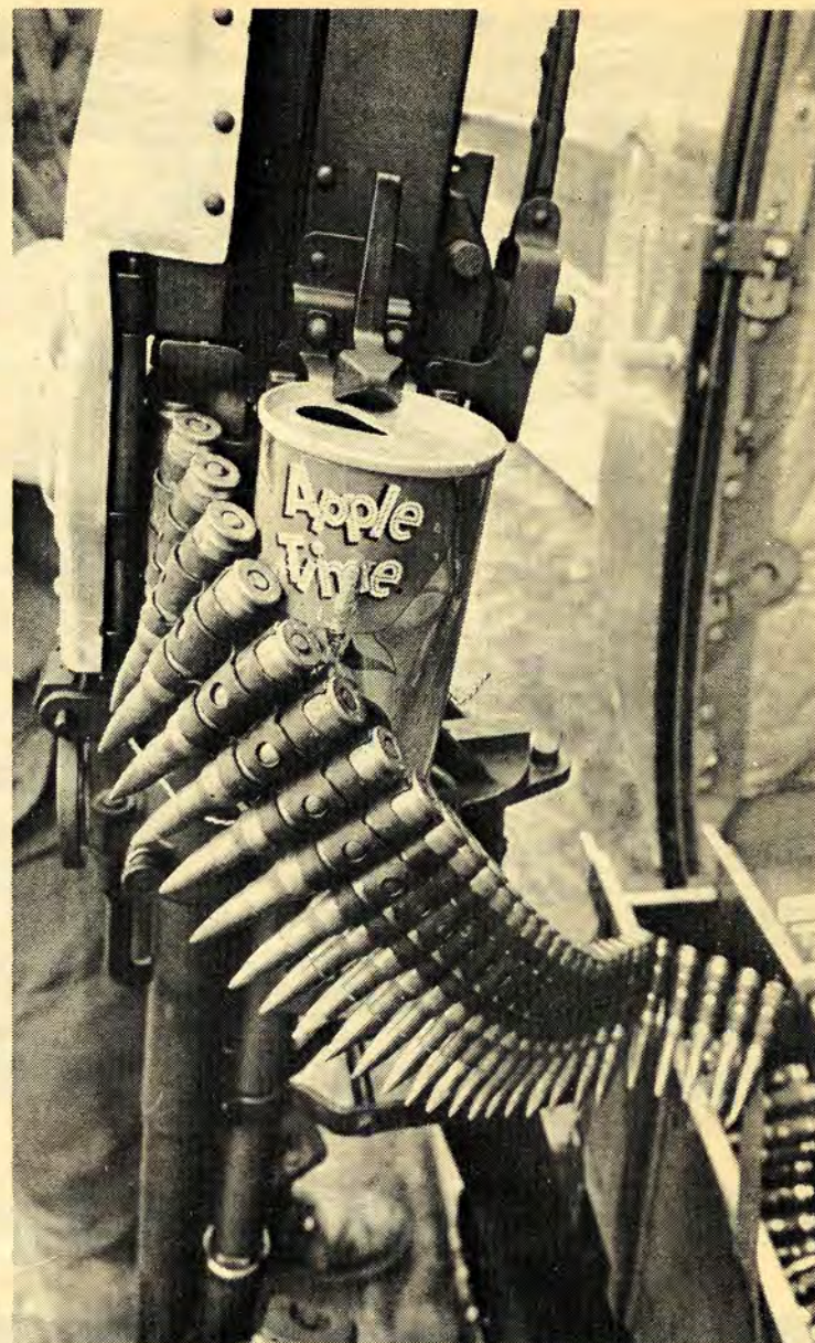
INGENUITY AT WORK —The idea of using a can, such as this apple juice can, to insure that the M-60 machinegun feeds properly is not new to soldiers in Vietnam. Somehow such ideas catch on quickly—and each person who tries it likes to think he came up with a new innovation (US ARMY PHOTO BY 1LT V. KENT FLANAGAN)
