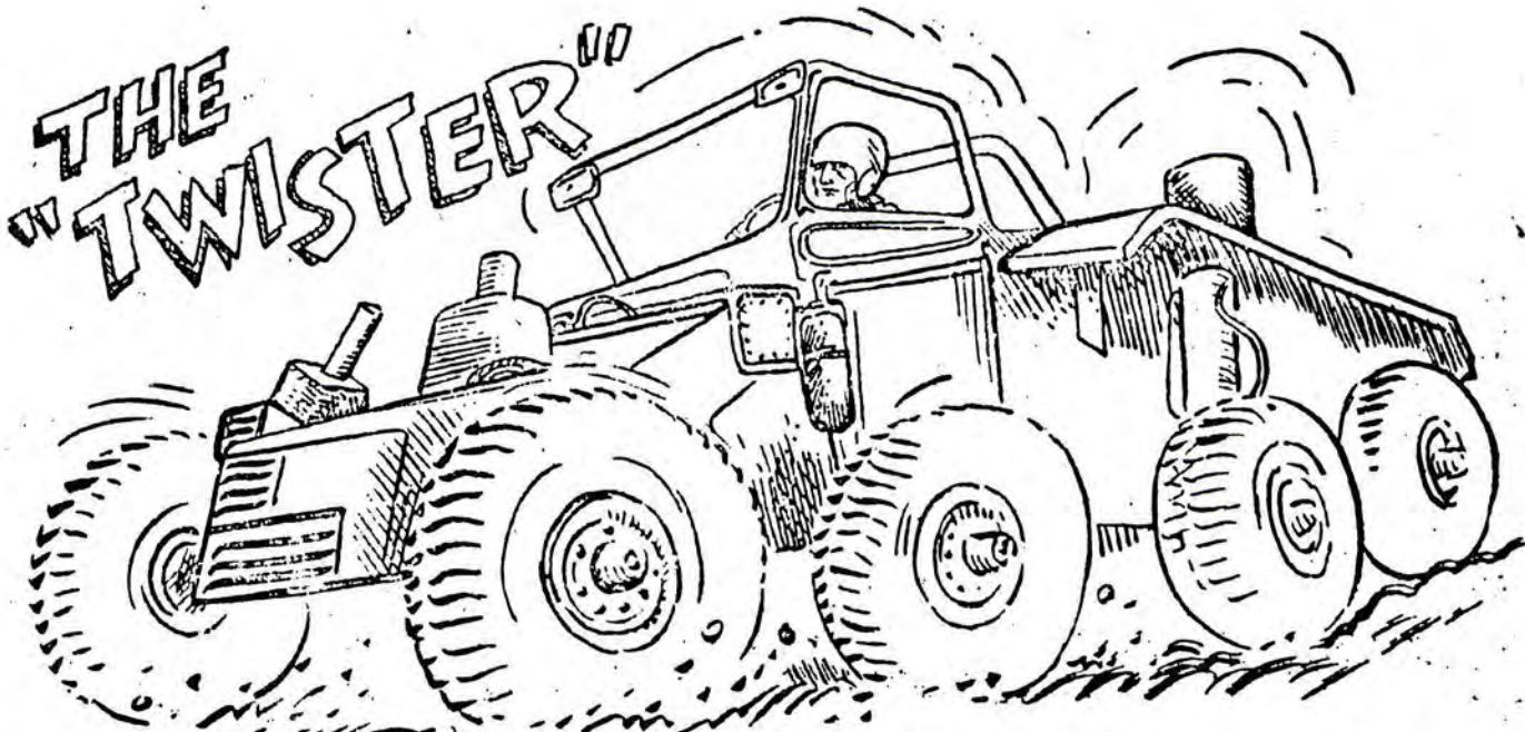
The "Twister" is the U.S. Army's new eight-wheel-drive vehicle that can move at high speed over rough ground where even jeeps and tanks can't go. The five-ton vehicle has two main body sections joined by a pivotal yoke that allows each unit freedom of movement while all eight wheels remain on the ground.
