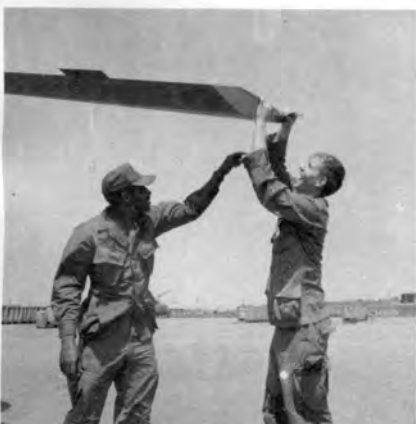
Pilot: M.E. Groce. Crewchief: Hines : Tracking UH1 Main Rotor
