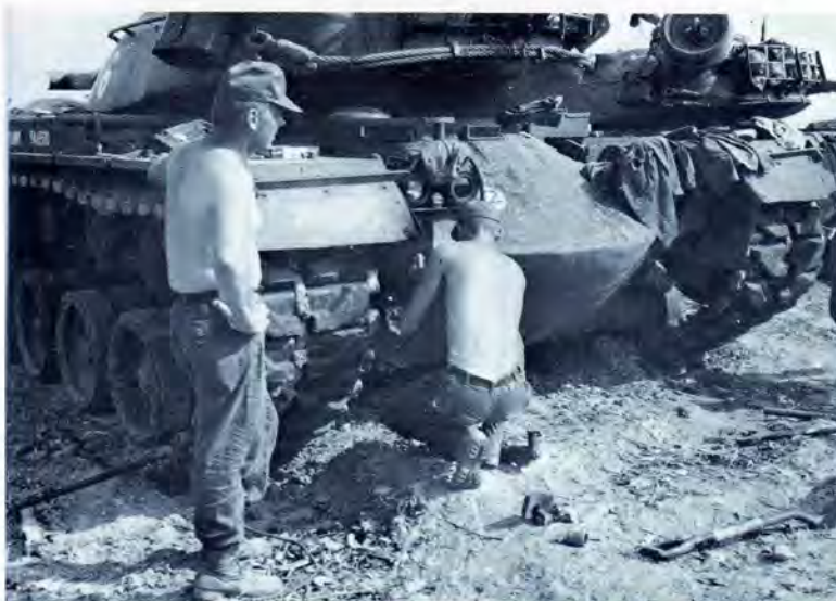
M48 tank tread undergoes repair at 69th Armor Battalion.
