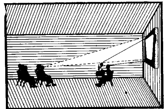
bottom of screen should be above student eye level
