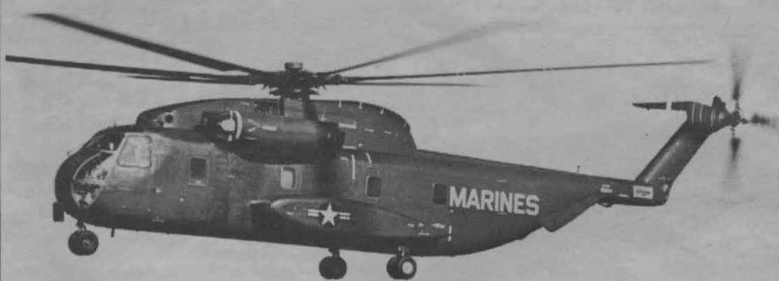
The Sikorsky CH-53A, the free world's most powerful heavy assault helicopter. The CH53 on a normal military mission can deliver over four tons of cargo at a cruising speed of over 170 mph. The helicopter can accommodate 38 fully equipped Marines. It has a combat operating radius of a hundred miles.
