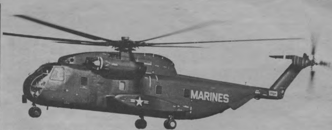
The Sikorsky CH-53A, the free world's most powerful heavy assault helicopter. The CH53 on a normal military mission can deliver over four tons of cargo at a cruising speed of over 170 mph. The helicopter can accommodate 38 fully equipped Marines. It has a combat operating radius of a hundred miles.
