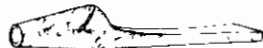
Drive Punch: Cuts holes in the thickest leather. Drive with a wooden mallet against a hardwood surface.
