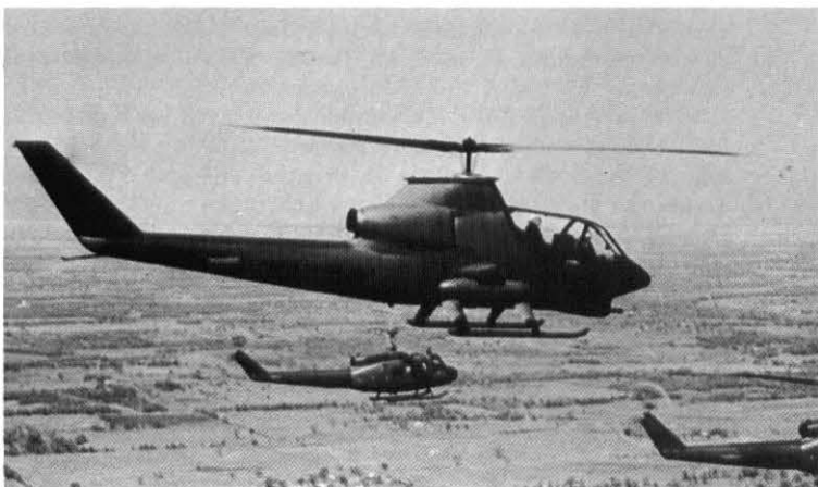
A HueyCobra gunship introduced in October 1967 flies alongside an older UH-1D. The chin turret is directed toward its target by the pilot turning his head. Photo by 1st Aviation Brigade-IO.
