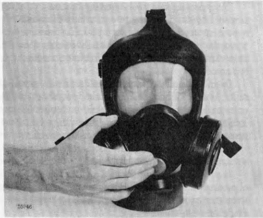
Figure 9770-13. Correcting sticking outlet valve, with cover partially removed.
