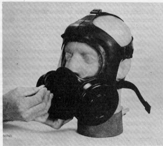
Fig. 9770-14. Removing canister; roll back apron.
