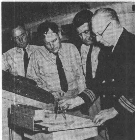
NIGHT PLOTTING is made easier by fluorescent maneuvering board demonstrated for deck officers in USNS Rose by inventor, LCDR Arthur J. Fraser, USMS, Electronics Instructor at U. S. Merchant Marine Academy. Placed next to radar set, the board is illuminated with ultraviolet light. Plotting sheets are printed in luminous ink. Dividers and protractors also are luminous. An identical maneuvering board is being tried out in USNS Kelley .
