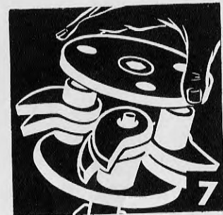
7 Place Round Hole Top Plate on top of the 3 Long Spacer Pins.
