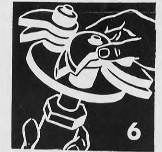
6 On the 3rd Spacer Pin, place 1 Large Spacer and then 2 Chipping Fingers.
