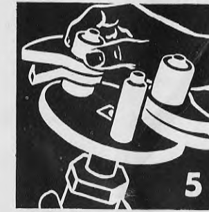
5 On next Spacer Pin place 1 Short Spacer, 2 Chipping Fingers and 1 more Short Spacer.
