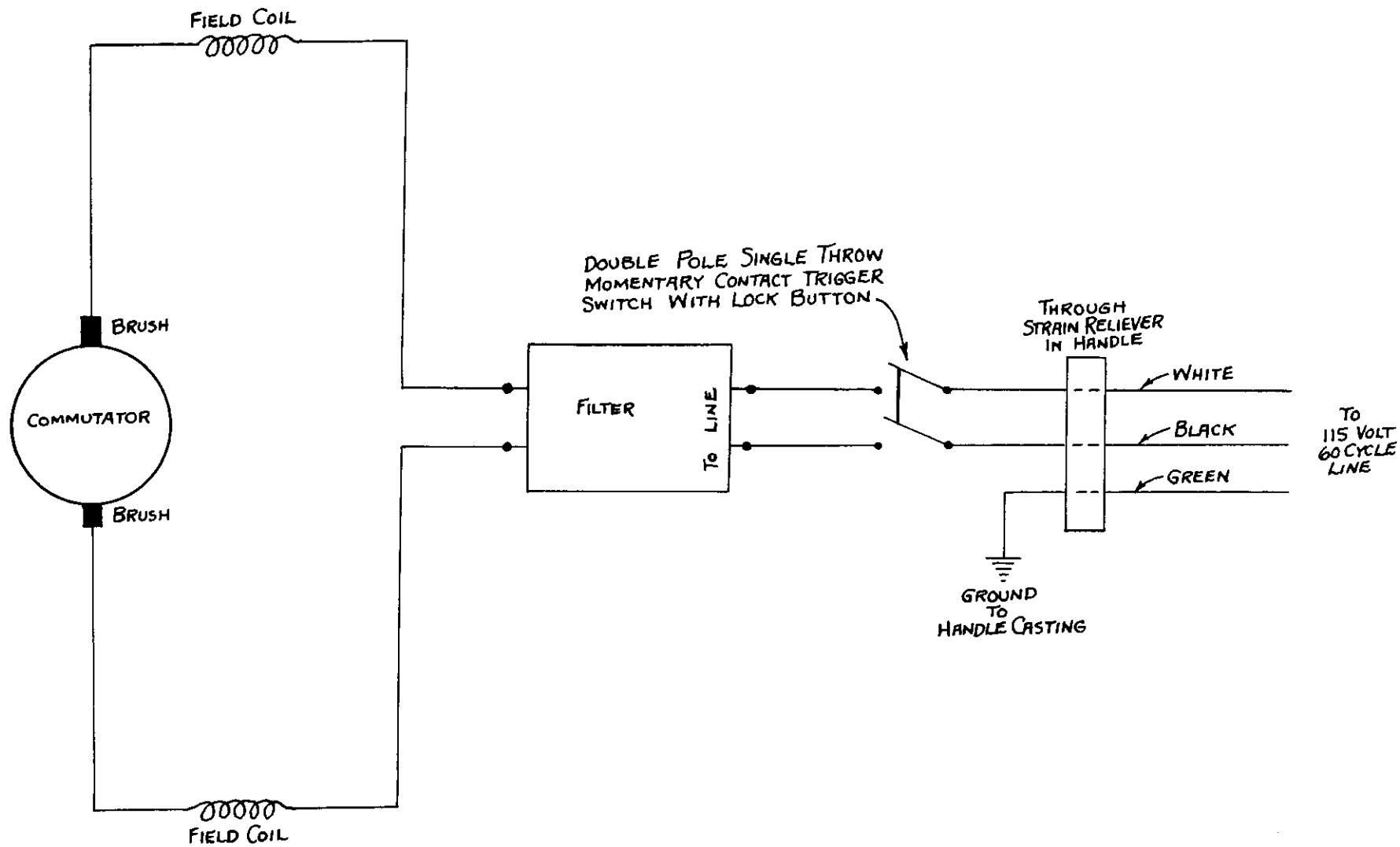
WIRING DIAGRAM FOR SCALING & CHIPPING TOOL
