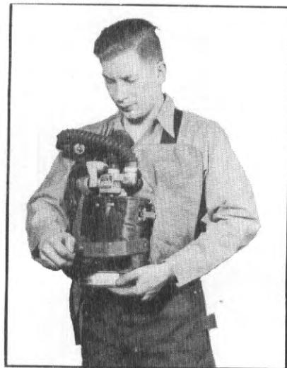
8. Slip on facepiece and adjust head straps to fit face and head size of individual.
