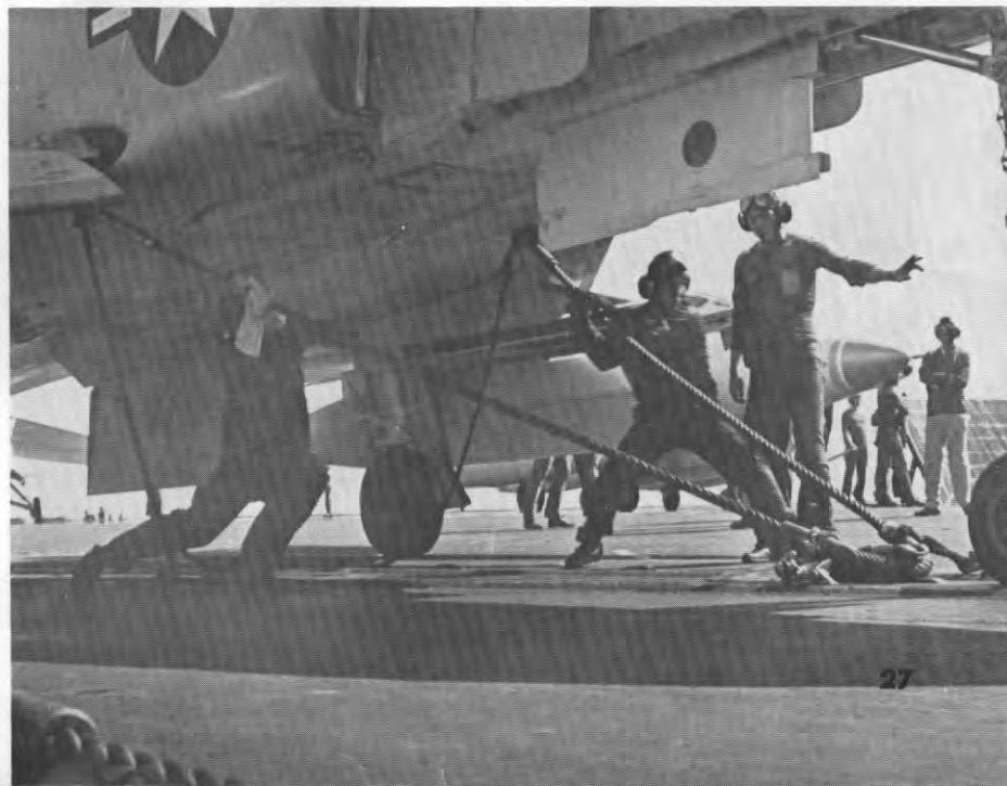
ON THE MARK —Catapult's water brake operator keeps close, close check. Rt: Bridle tension is tested prior to launching.
