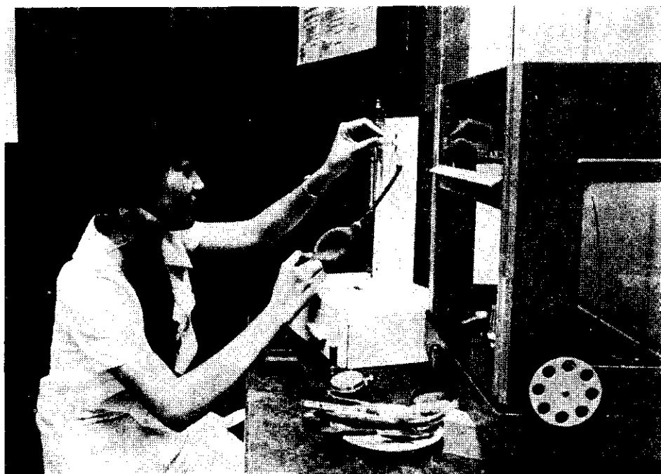
Laboratory technician Nguyen Thi Kim Hoa tests cement's kneading periods.
