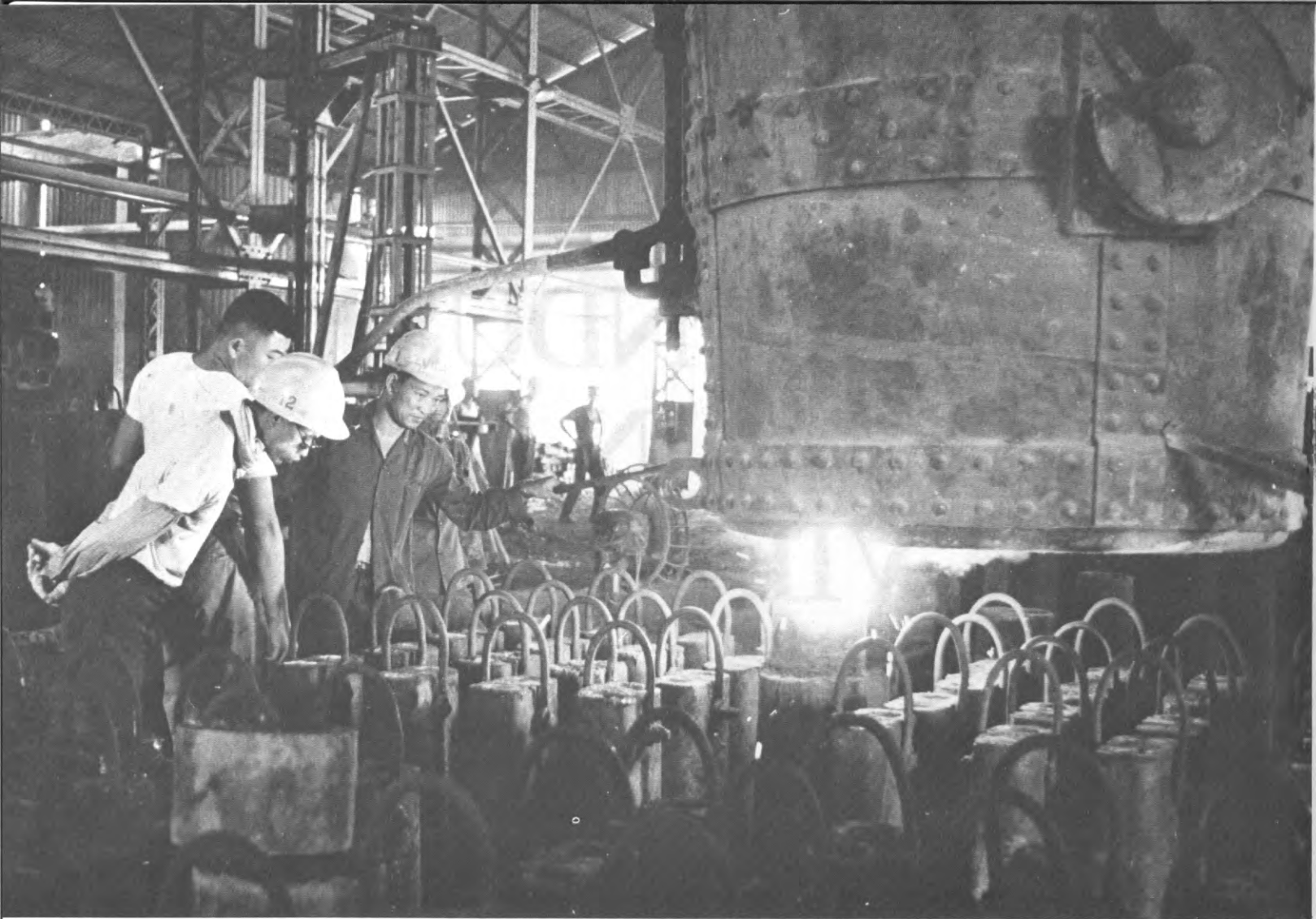
Workers at VICASA Steel Mill handle the enormous molten steel bucket with care as liquid metal flows from an open cock into ingot molds.
