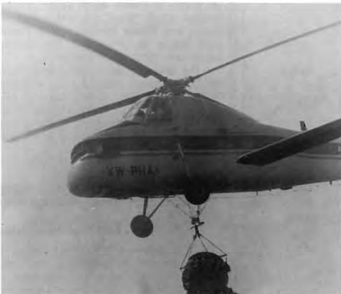
10. Close-up of airborne XW-PHA with slung engine.
