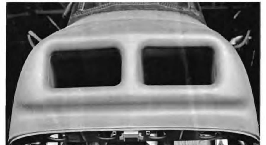
9. Close-up view of the Twin-Pac engine intake air ducts.
