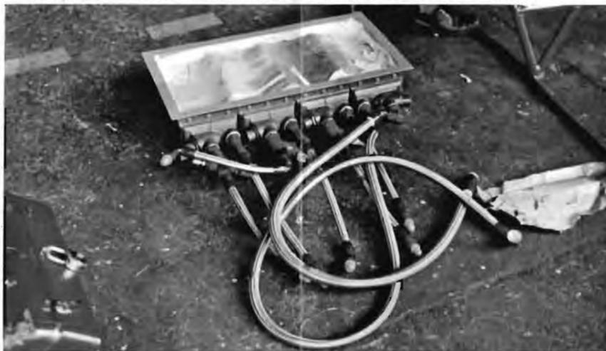
6. Four S-58T oil coolers combined into a single package. One cooler is used for each of the two turbines; one for the combining gearbox, and one for the angle change gearbox.
