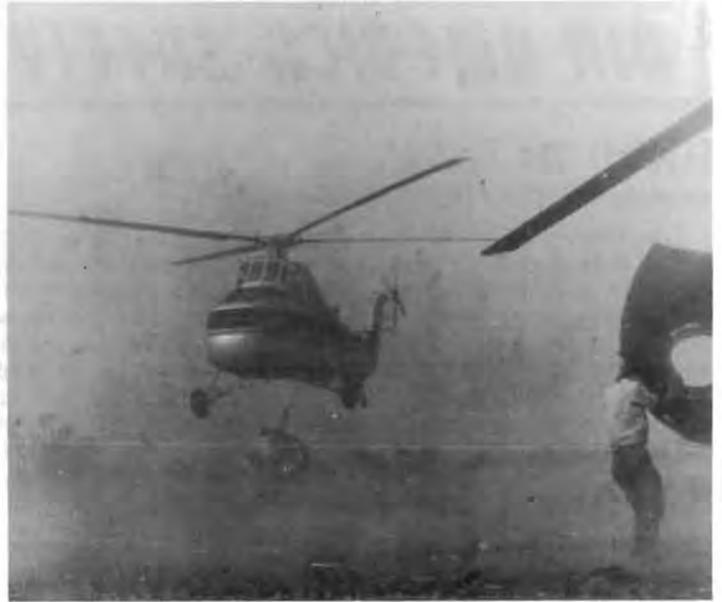
7. H-73's engine being attached to XW-PHA's sling.
