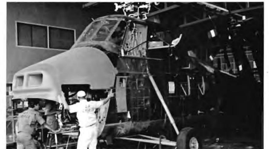
8. An S-58T begins to take shape in Air America Udorn shops. Twin-Pac conversion nose and intake ducts are installed.
