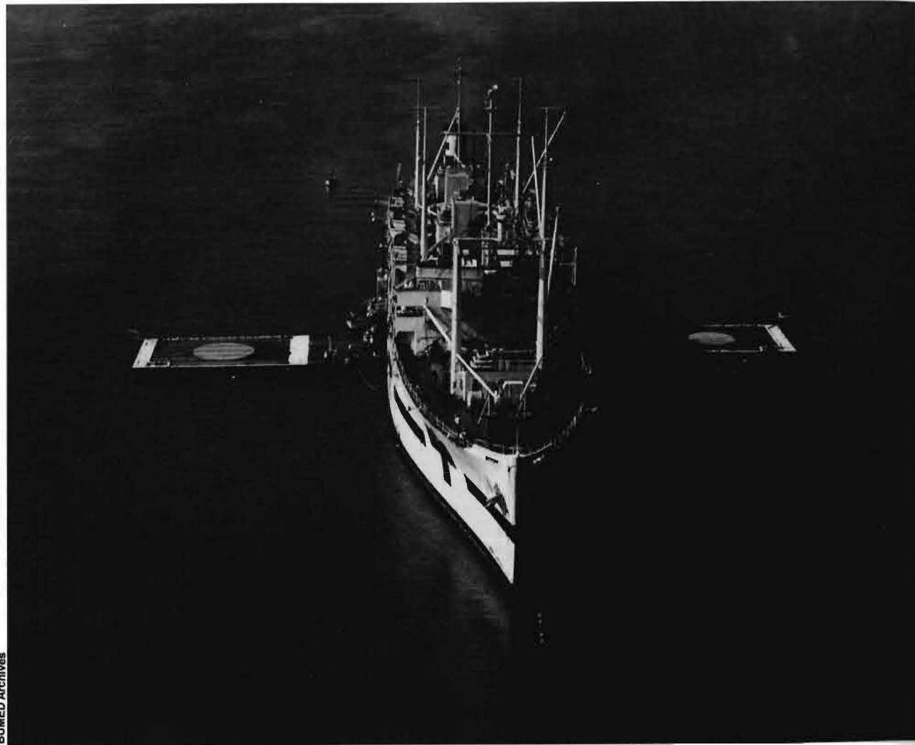
(Above left) USS Haven with its newly installed pontoon landing floats. Inchon, July 1952. (Opposite top) USS Consolation . Inchon Harbor. (Below left) Securing bridge pontoon to Haven's port side. July 1952. (Below opposite) Bell HTL-4 aboard one of Haven's pontoon landing floats. July 1952.
