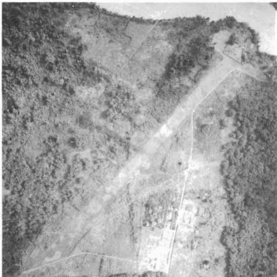
CAY GAO, VIETM YT300254 11°05'N 107°06'E PVT 230 26(EARTH) 04/22 98' wide (C-123) AERODROME REMARKS - Overgrown.
