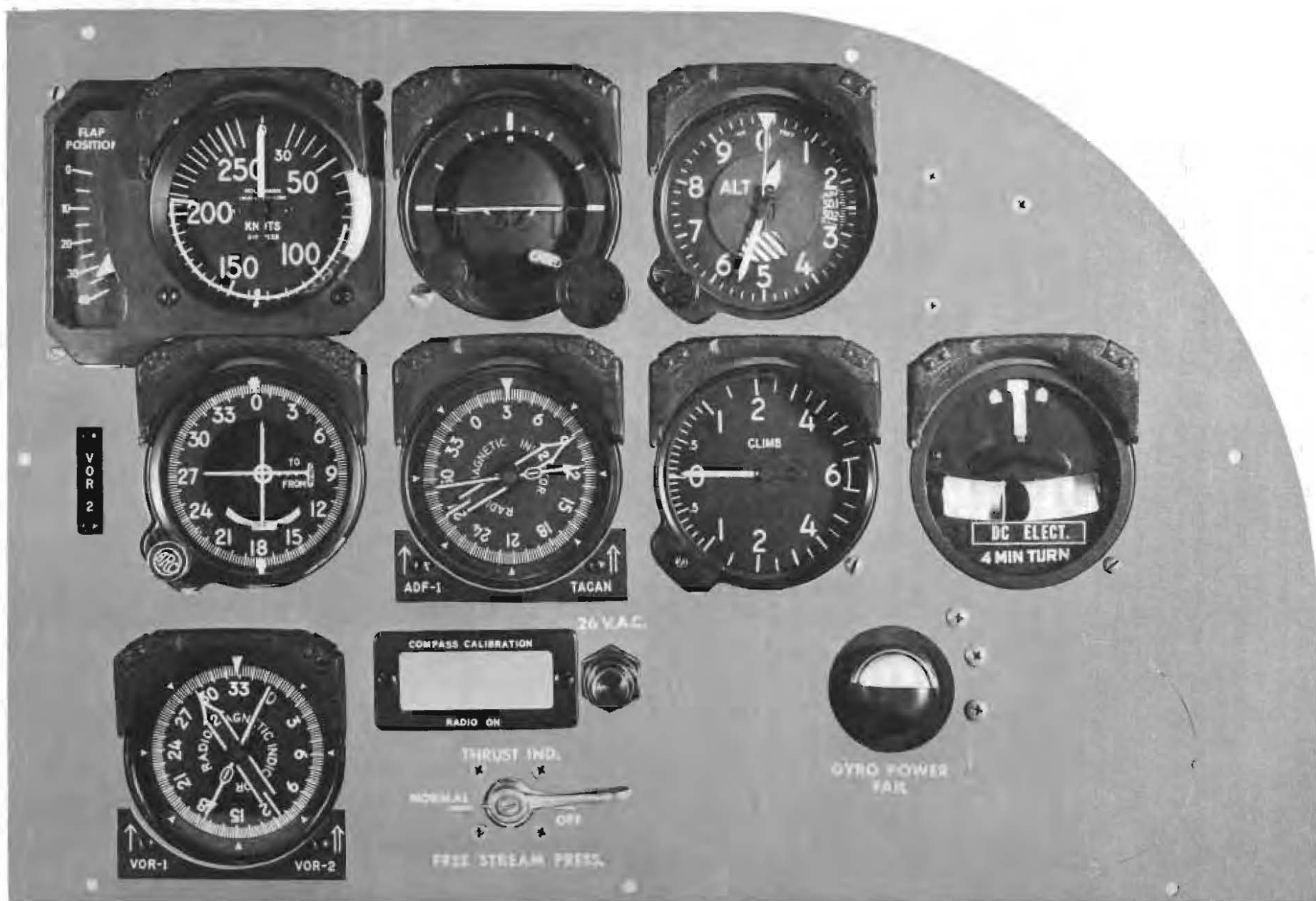
Figure 1-16 Copilot's Instrument Panel - Typical
