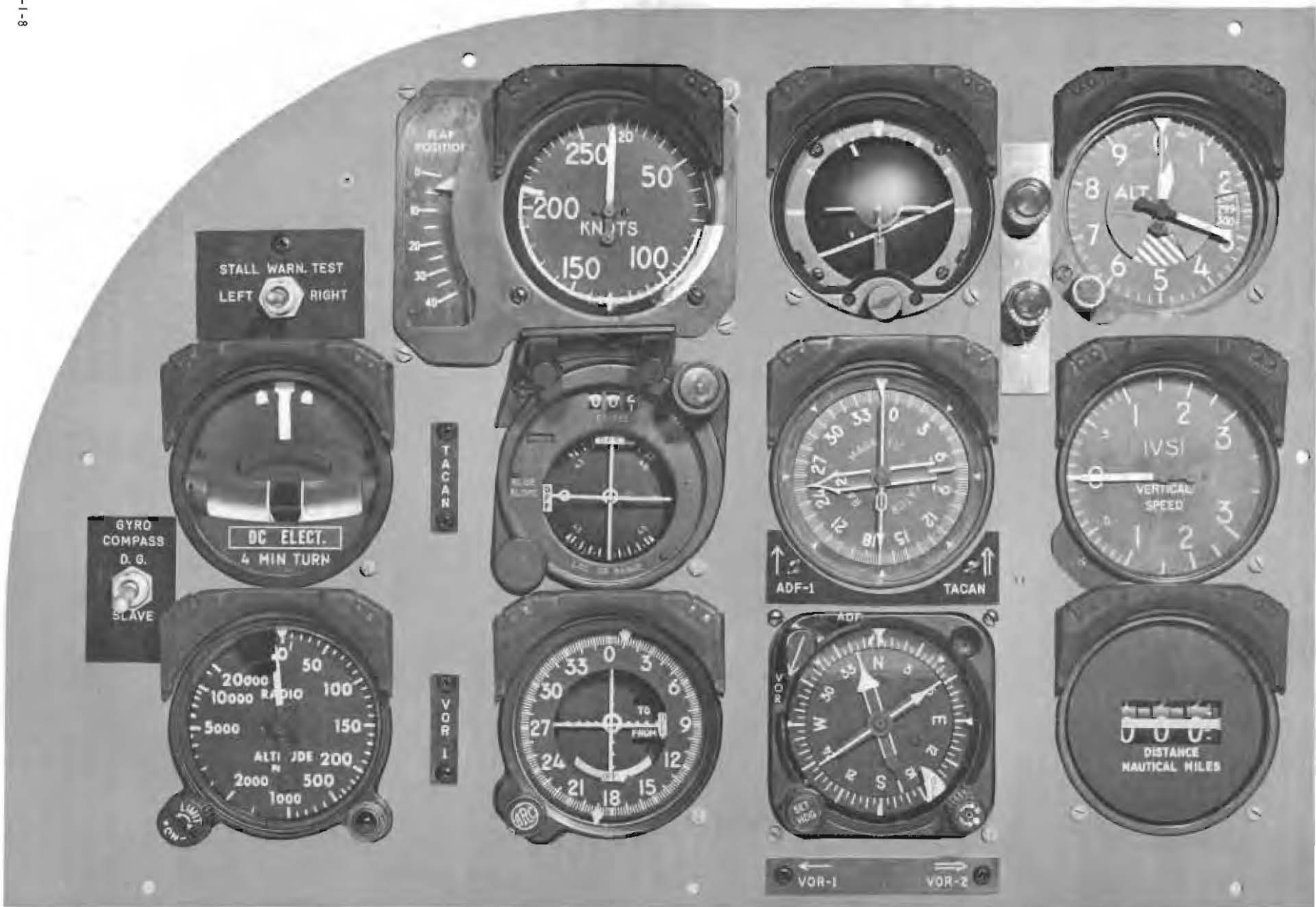
Figure 1-15 Pilot's Instrument Panel - Typical
