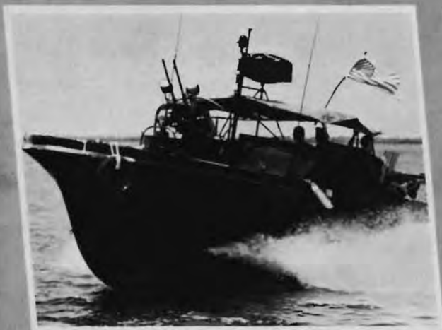
USN Patrol Boats, River (PBR) are made of fiber glass and are guided by twin jets of water. In motion, they draw as little as nine inches.
