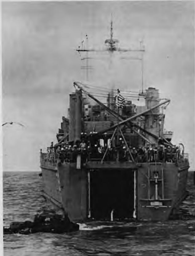
STERN LOOK —An amphibious landing craft prepares to enter well deck of the new style LST.
