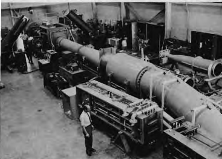
NOL hypersonic wind tunnel attains speeds up to Mach 10.
