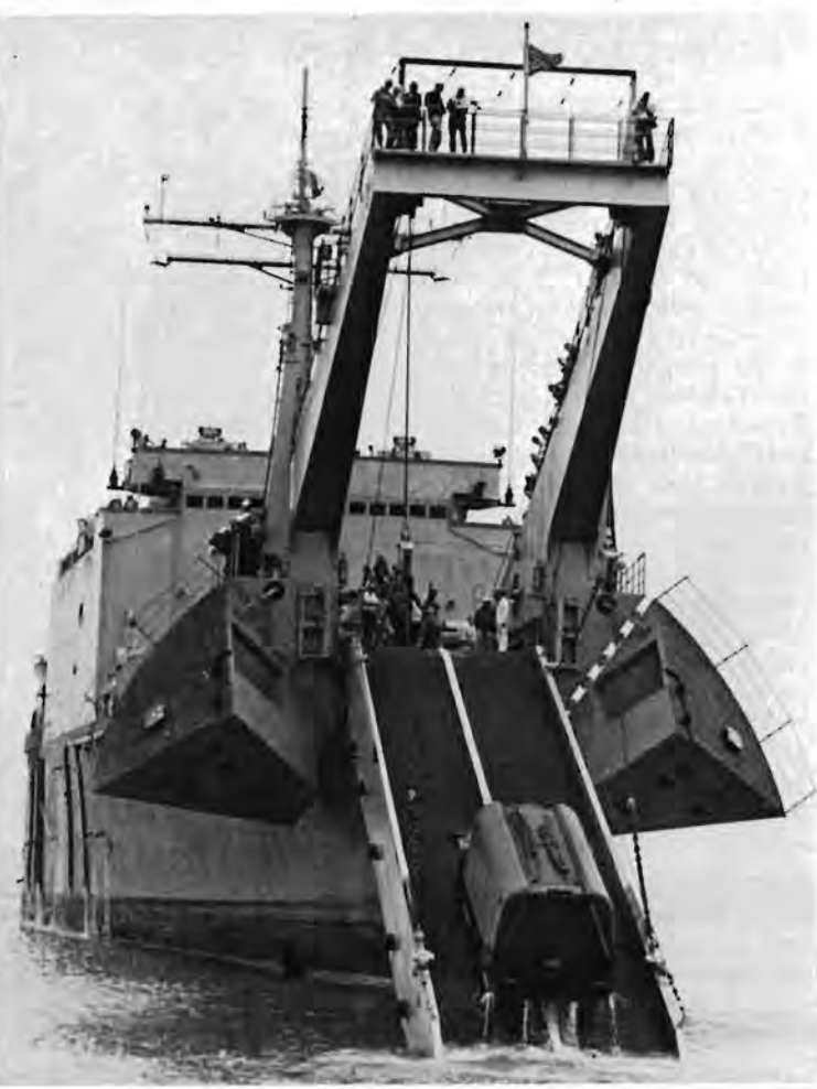
UPHILL CLIMB —Truck tests traction of bow ramp of new LST. Below: Tank landing ship USS Newport (LST 1179) lies at anchor off coast of Virginia. Rt: Landing craft emerges from stern during evaluation tests on underway launching.
