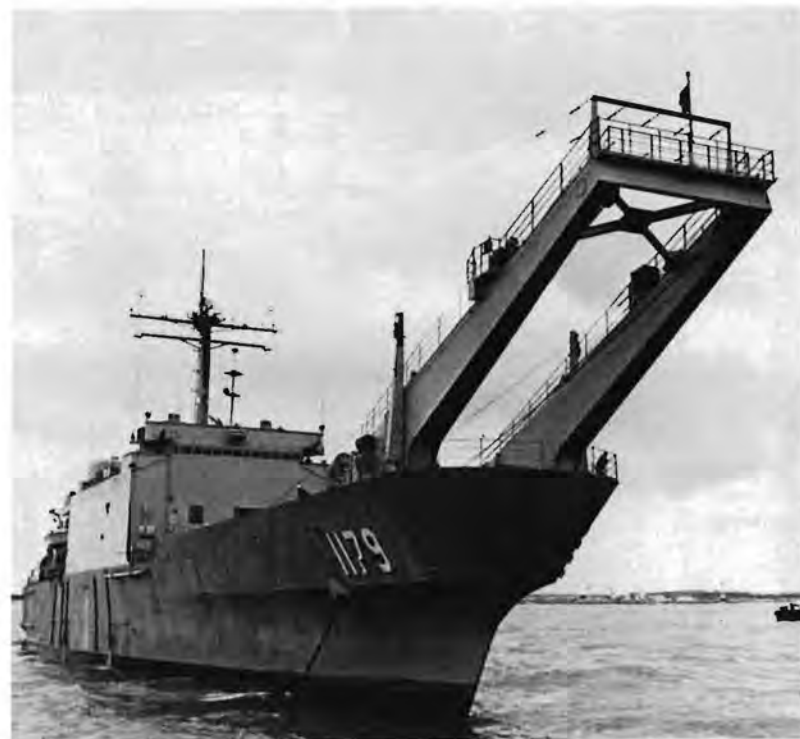
UPHILL CLIMB —Truck tests traction of bow ramp of new LST. Below: Tank landing ship USS Newport (LST 1179) lies at anchor off coast of Virginia. Rt: Landing craft emerges from stern during evaluation tests on underway launching.
