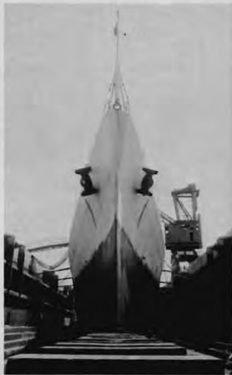
Left and above: Standing in her drydock at the Pakistani Naval Shipyard, the USS Valcour is sandblasted in preparation for a new coat of paint.
