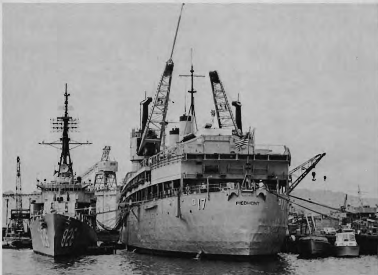
Above: The Seventh Fleet destroyer tender USS Piedmont (AD 17) renders repair and maintenance service to the destroyer USS Agerholm (DD 826). Below left to right: (1) An EM3 rewinds a section of a 340-pound saltwater circulation pump. (2) A Navyman regulates Piedmont's number two AC generator. (3) Oil bond sand is packed to make a mold in the ship's foundry. (4) An MR3 parts off a piece of stock on one of Piedmont's turret lathes. (5) Lens is polished in the optical shop. (6) A pantograph machine is used to engrave bakelite signs.
