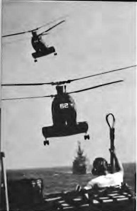
■ Underway replenishment of Navy ships at sea is a daily occurrence off Vietnam. The amount of beans, bullets and black oil needed to keep 60,000 men working, approximately 50 combatant ships operating and 500 aircraft flying is considerable. Ships still must be carefully maneuvered side by side to deliver fuel and other supplies from supply ship to combatant, but the rate of transfer of hard goods from ship to ship has tripled, thanks to the addition of the helicopter.
