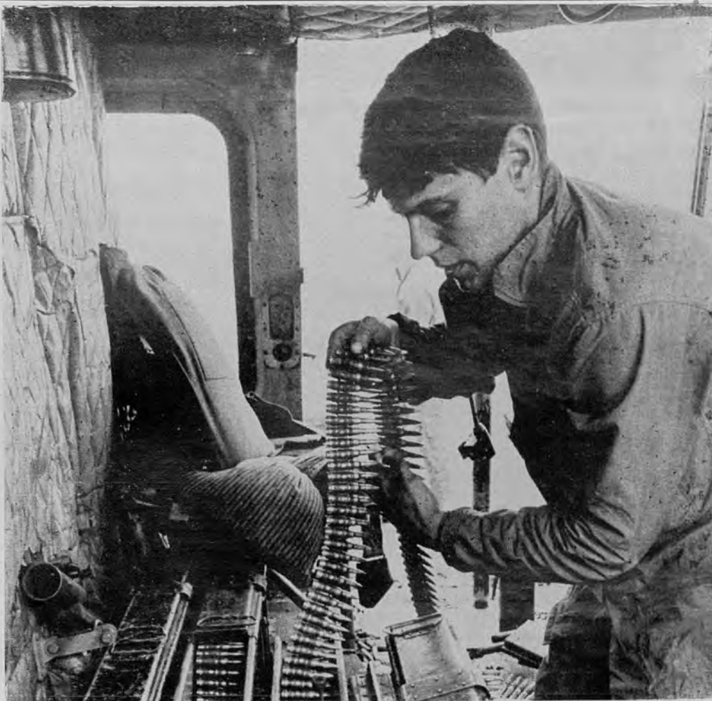
LOADING —Airman Robert Nunes, loads the ammunition box for the externally-mounted M-60 flex-guns. There are two ammunition boxes for each set of flex-guns.
