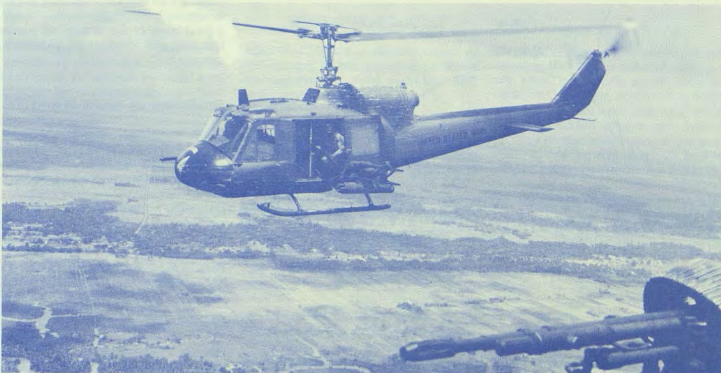
UH-1B of HAL-3 the U.S. Navy "Seawolves", who operated the Huey in the gunship role, beginning in 1966. Note that this B model has been modified with the larger C vertical tail surface. (U.S. Navy)
