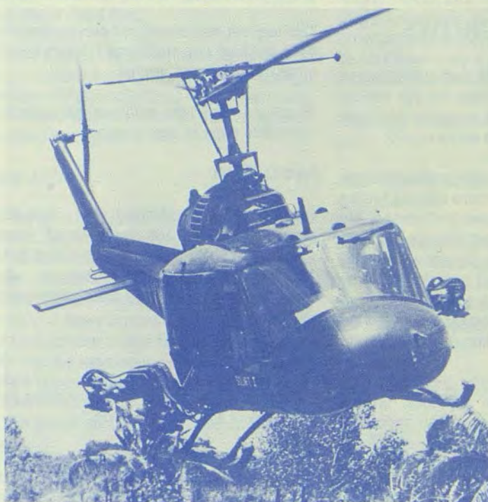
UH-1B of HAL-3 the U.S. Navy "Seawolves", who operated the Huey in the gunship role, beginning in 1966. Note that this B model has been modified with the larger C vertical tail surface. (U.S. Navy)
