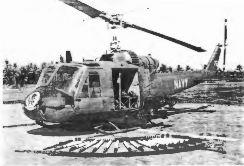
A Seawolf Huey and the various weapons it carried. Not shown are the .30 and .50 caliber machineguns carried by some ships to counter the VC's increased anti-aircraft defenses which began to be encountered in the mid-1960s. The Seawolf insignia is carried on the nose and NAVY on the Boom. Some helicopters carried the words UNITED STATES NAVY in black on the boom early in the war. (US Navy via Cressman)
